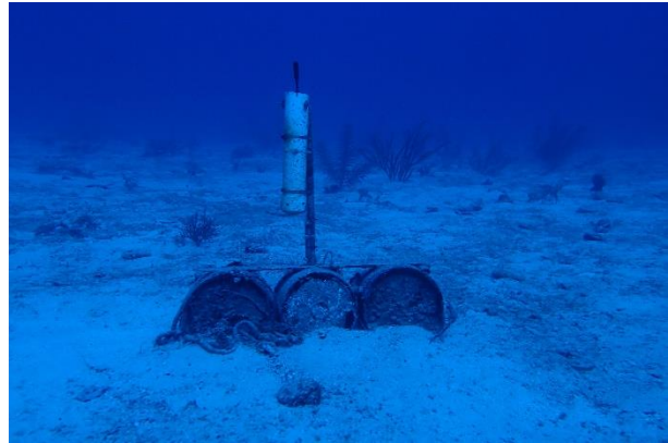
Figure 10 Hydrophone installed at FSA site (Credit: COBI).
