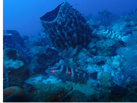
Figure 8 A Nassau grouper with laser points on its lateral surface. Still frames are extracted from video footage and are used to extrapolate fish size. (Credit: A.Tewfik/WCS).
