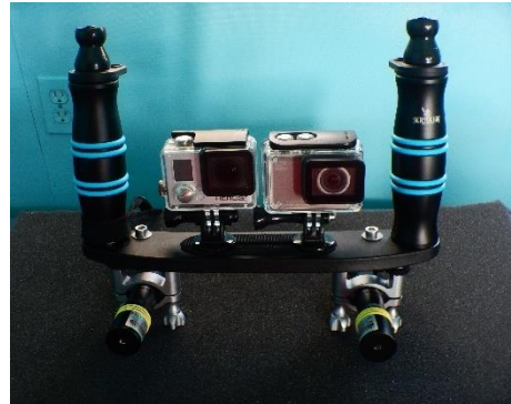
Figure 7a Laser caliper array used by WCS Belize (Credit: A.Tewfik/WCS).
