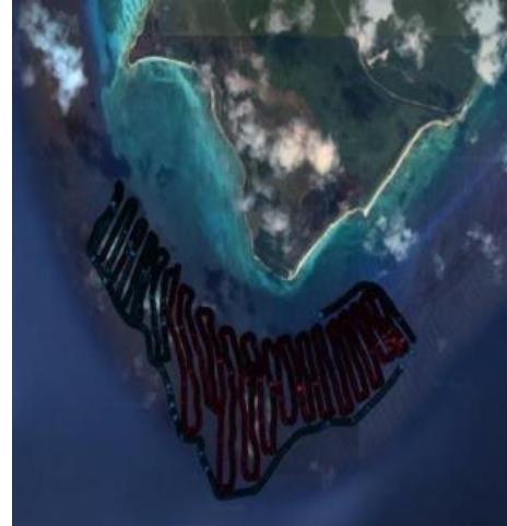
Figure 5 Example of transects to collect bathymetric data (Credit: COBI).
