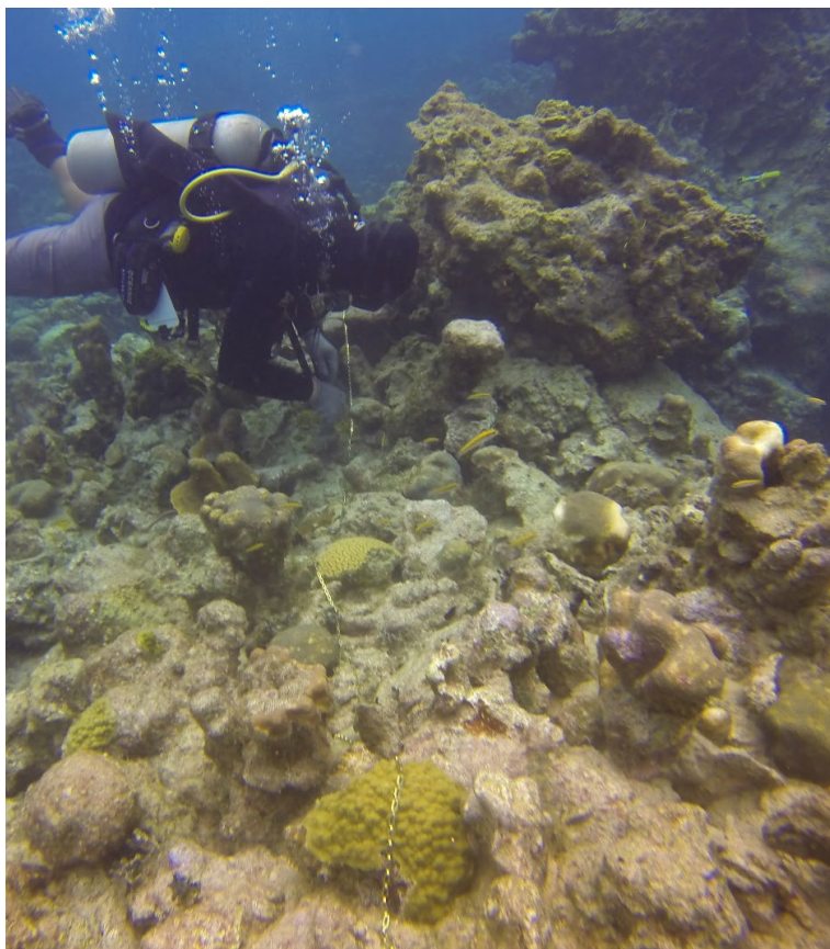
Figure 18. Laying out weighted chain (gold-colored links in image) to measure rugosity.
