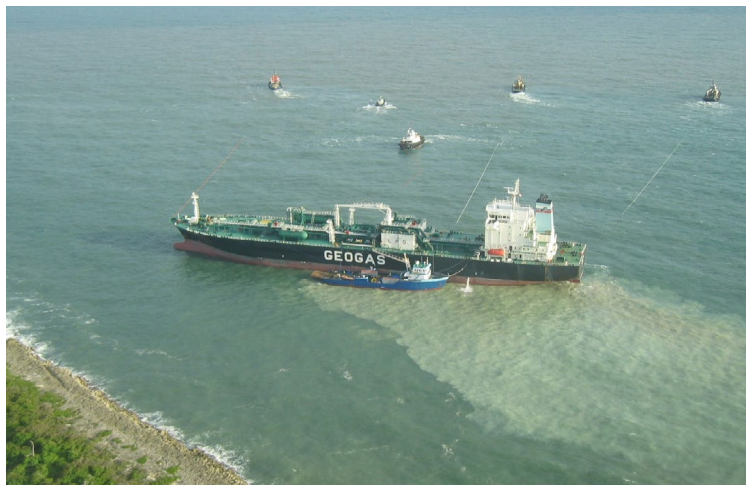
Figure 12. Tugboats attempting to salvage a stranded liquefied petroleum gas carrier.
